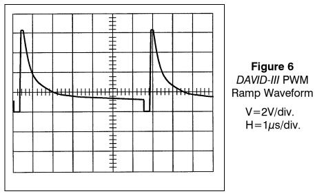
This ramp runs continuously at a 152kHz rate. It is applied to one input of a comparator, and a DC voltage derived from the input signal is fed to the other comparator input. The comparator output is the duty-cycle-modulated squarewave that 'chops' the program audio signal.
